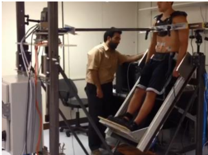
Figure 3.7: Platform Rising During Stress Relaxation Test (Photo provided by the HMB Lab at the University of Kentucky)
